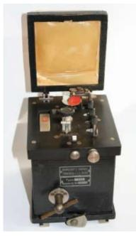
TELEFUNKEN DEVICE – This large, slider type, clockwork device was made by Gesellschaft f.drahtlose Telegraphie m.b.H. Berlin (Telefunken) during World War I. It was constructed for reception of damped and continuous waves and for testing of transmitters and receivers for continuous waves. The wheel on the left indicated by an "O" on top is a timer that runs about two hours. This set is a great novelty and now the oldest set in my collection. (Erwin Macho – Vienna, Austria)
