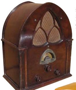
Atwater Kent Model 84 - This 1931 receiver was the first cathedral radio that Atwater Kent produced. It is a 6-tube Hetrodyne circuit with the new, (then), screen-grid tubes. It tunes the broadcast band only. (Dave Crocker - Mashpee. MA).
