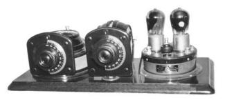
ATWATER KENT MODEL 3925 - This breadboard was one of the first receivers Atwater Kent manufactured. It was sold in 1923 for \$23, and consisted of a 2-tube TA unit (detector/amplifier), a coupled circuit tuner, and a variomenter. (Wally Worth—Wollaston, MA)
